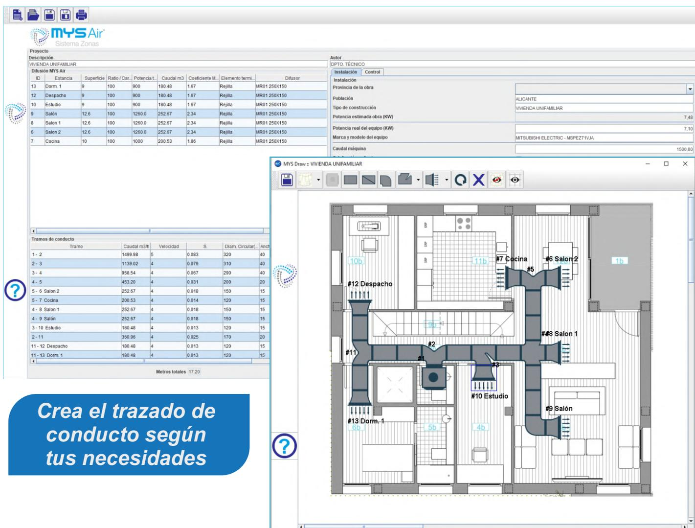
The screenshot displays the MYS Draw software interface. The top window shows project details for 'VIVIENDA UNIFAMILIAR' with a table of room data and a summary of ductwork. The bottom window shows a detailed duct layout diagram for the same unit, with rooms labeled and duct paths numbered.
